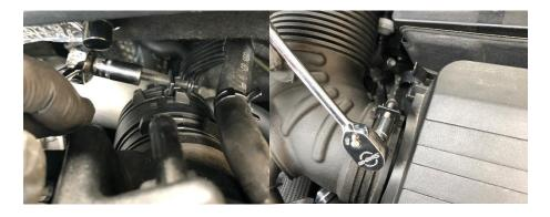
3. To remove the airbox undo the 3 x 10mm bolts and then push in the 2 pins holding on the scoop to the front panel by using a small screwdriver or similar and then pull the pins out. The whole assembly can then be lifted out of the car.
