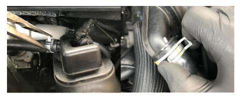
2. Undo the hose clamps at either end of the induction pipe there are undone using a 10mm socket, once undone the induction pipe can be removed from the car.
