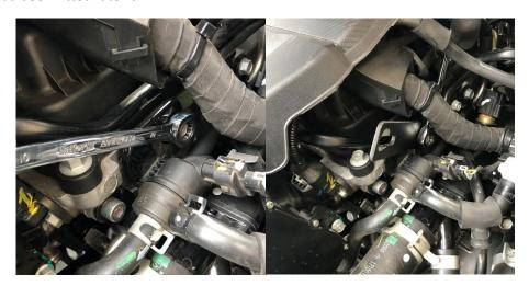
6. Install your new AIRTEC Motorsport shield by firstly placing the supplied spacer on the right side of the engine bay where the original front right airbox bolt was threaded into (see picture below) and then place the induction shield into location using a 5mm Allen key and the provided M6 x 35 bolt for the right hand side, M6 x 12 for the rear mount and re-use one of the 10mm bolt from the cold air feed block to attach the shield to the front panel.
