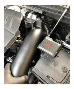
8. Using the supplied M6 x 12 dome headed bolt and washer mount the bracket that was fitted to the block earlier to the boss on the side and tighten to hold the pipe securely to the bracket, leave the bracket itself still slightly loose at this point so the pipe can be positioned correctly once the filter is on.
