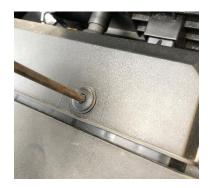
4. Undo and remove the cold air feed block that is attached to the front panel shown in the photo below, retain 1 of the bolts as this will be reused when fitting the new induction shield.
