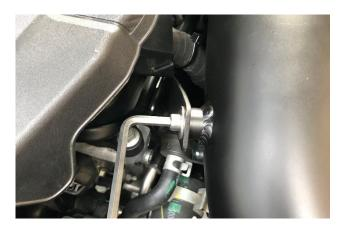
9. The 2 breather hoses at the back can now be reconnected reusing the original clips along with the hose that connects onto the front.
