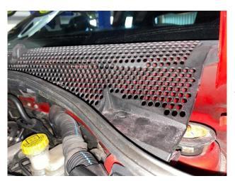
lift the scuttle and disconnect jets from the to remove.
