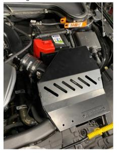
12. Remove the 10mm bolt from the slam panel (as shown) and slide the AIRTEC Motorsport mounting bracket into the front of the air box and then secure in place using the provided M6 bolts and washers. You can then reinstall the 10mm bolt through the bracket into its original location.
