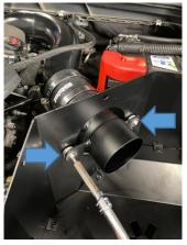
10. Remove the sensor from the original air box and reinstall it into the new pipe, securing it in place using the supplied bolt and clamp. Then attach your AIRTEC Motorsport air filter using the jubilee clip supplied.
