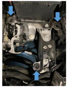
6. Install the three locating pins to the lower piece of the air box using three of the M6 bolts and larger Mudguard washers provided.
