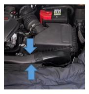
4. With the cold air feed separated, remove the standard air box by carefully but firmly pulling it up off its rubber mountings and remove from the engine bay.
