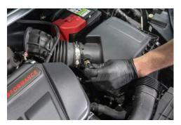
2. Loosen the jubilee clip and remove the hose from the air box by carefully but firmly pushing it back.
