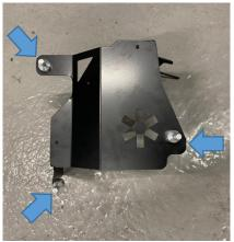
7. Attach the back piece of the air box to the lower piece using three of the M6 bolts and washers. Start with the left-hand bolt first but do not fully tighten. Then line the middle bolt up but do not fully tighten before lining the right-hand bolt in place. Once all bolts are engaged, fully tighten them.
