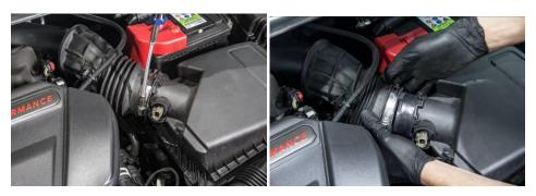
3. Disconnect the cold air feed from the air box by pushing the securing tabs using a plastic trim tool or flat-bladed screw driver. Please note: If using a flat-bladed screw driver, we recommend covering the end with masking tape to prevent scratching the air feed.
