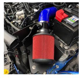
1. Start with removing the original airbox by unplugging the IAT (inlet air temperature) sensor and then using a flat blade screwdriver or trim removal tool to remove the grey plastic tab or cut the tie around the cable as the clip will not be reused when fitting the Airtec induction kit (see pictures below) from the airbox lid and then use the screwdriver to remove the black clamp (see pictures below) so that the cable is now free of the airbox.
