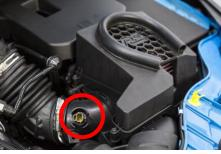
3. Undo 1x 10mm bolt, 1x 8mm bolt and 2x jubilee clips on the original crossover pipe and remove
