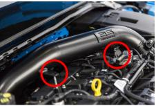
7. Once happy with the position of the crossover pipe, install MAF sensor onto new crossover pipe and secure jubilee clips onto straight reducer
