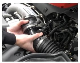
5. Now remove x2 10mm bolts securing airbox air guide, after removing these bolts you can also unclip and remove the seal from the bumper scuttle using a trim tool.
