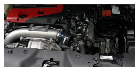
9. Install the heatshield and secure in place using the supplied M6 x 12mm fixings with washers.
