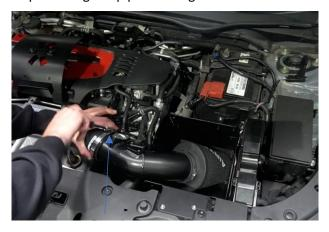
11. Remove x2 10mm bolts securing vacuum line feed to OEM pipe work as you will need to reinstall vacuum line feed into your new pipework.
