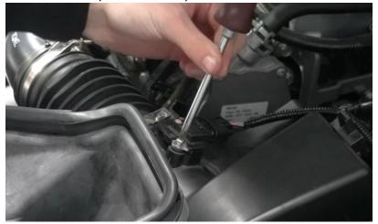
2. You can now loosen the jubilee clips securing pipework in place by using either a 5mm socket or a Philips head screwdriver.
