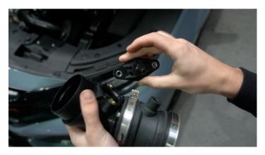
12. Now reinstall the vacuum line feed into your new pipework reusing the x2 10mm bolts then reconnect the vacuum line.
