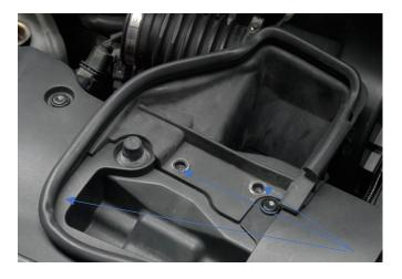
6. At this point we can now fully remove the air guide and seal from the engine bay.
