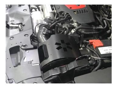
14. Finally reinstall your MAF sensor using the supplied M4 x 12mm and check everything has been secured correctly.
