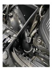
8. Remove the MAF sensor from the original pipework by removing the two Torx bolts using a T15 socket. Now install the MAF sensor into your new pipework and secure in place using the provided M4x12mm Socket Head bolts with Pan washers and reconnect the wiring.
