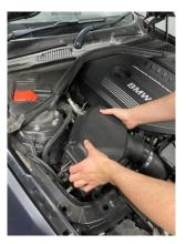
3. You will now have access to release the jubilee clip at the bottom of the hose, using a 6mm socket or flat-bladed screwdriver. Once the clip has been released the hose can be removed from the engine bay.
