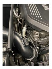
9. Finally, install the air filter onto the pipework and secure in place using a flat-bladed screwdriver.
