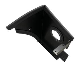
6. The heat shield can be installed into the engine bay. Once in place, reinstall the two 13mm bolts and the mounting post removed in Step 4 to help secure it in place. Now install the smaller support bracket to the tab on the strut tower behind the heat shield. Align the bracket with the allocated hole on the heat shield and secure using the provided M6x12mm Button Head bolts with Pan washers and Nyloc nuts.
