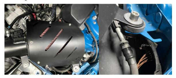
13. Reinstall the brace removed at the start and when happy with the position of the hardpipe fully tighten the original jubilee and bolt to firmly secure the induction kit.
