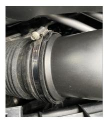
6. Pull up on the plastic bracket securing the plastic pipe to the front of the car to release the rubber fitting and then remove the rubber grommet and insert into your new AIRTEC motorsport hard pipe.
