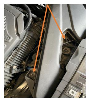
2. Now remove the 10mm bolt securing the air box inside the engine bay.
