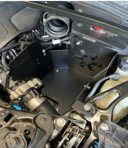
6. Now you can install your AIRTEC air filter with pipework into the engine bay by securing in place using the bracket attached to the back of the heatshield connecting to the pipework. This can be secured using supplied fixings then tighten the jubilee clips attaching the pipework to the hose.
